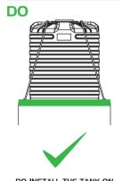
DO INSTALL THE TANK ON A FLAT, LEVEL BASE,
